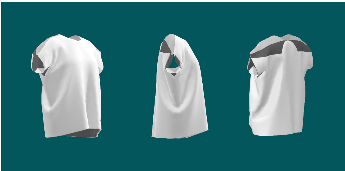
Figure 9. T-shirt iteration Three, showing expanding layers at shoulder and armhole (in light and dark grey) to enable fit and ease of movement. Only the side seams are needed to be sewn in this t-shirt, in contrast to the usual side, shoulder and armhole seams in a conventional garment..
