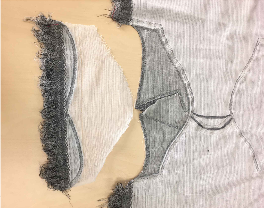
Figure 4. T-shirt iteration one, sleeve layer cut from body. Transparency of sleeve is caused by the low weft and warp density of the loom.
