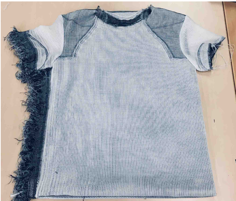
Figure 5. T-shirt Iteration One is sewn using a standard t-shirt construction sequence, side seams, shoulder seams and armhole. Auxiliary selvage shown as fringe on left side, this can be removed.
